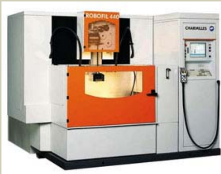
One of the two wire EDM's that produce parts around the clock
